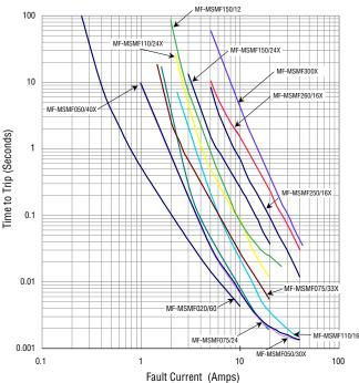
The Time to Trip curves represent typical performance of a device in a simulated application environment. Actual performance in specific customer applications may differ from these values due to the influence of other variables.
