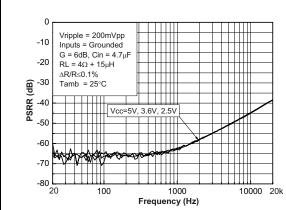
0 Vripple = 200mVpp -10 Inputs = Grounded G = 6dB, Cin =  $4.7\mu$ F -20  $RL = 4\Omega + 30\mu H$ ΔR/R≤0.1% -30 (dB) Tamb = 25°C PSRR ( -40 Vcc=5V, 3.6V, 2.5V -50 -60 -70 -80 1000 Frequency (Hz)
