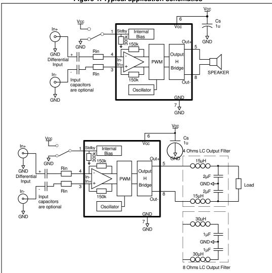
Figure 1. Typical application schematics
