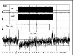
Figure 57. Startup and shutdown times
