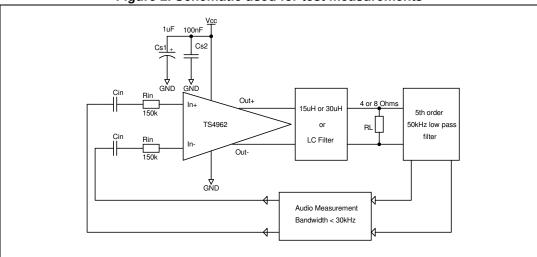
Figure 3. Schematic used for PSSR measurements
