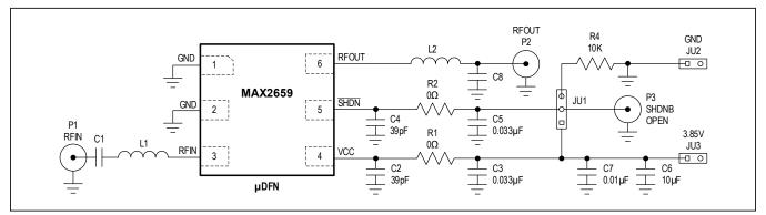
Figure 1. MAX2659 EV Kit Schematic
