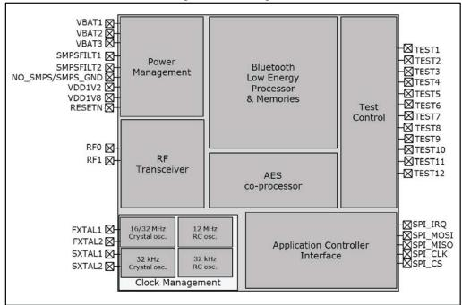
Figure 9: Block diagram
