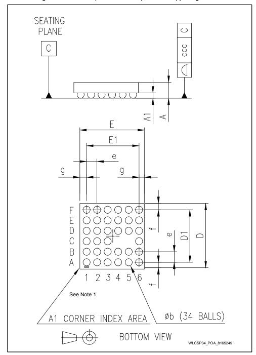
1. The corner of terminal A1 must be identified on the top surface by using a laser marking dot.
