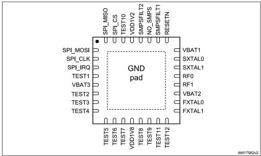
Figure 2: Pinout top view (QFN32)
