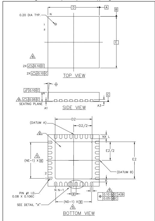
Table 20: QFN32 (5 x 5 x 1 pitch 0.5 mm) mechanical data
