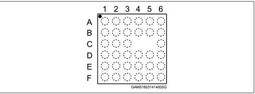
Note: Top view (balls are underneath).
