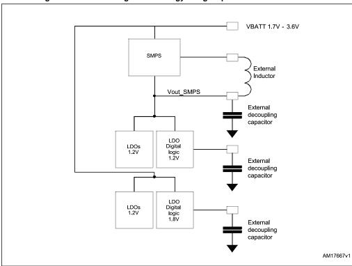
Figure 11: Power management strategy using step-down DC-DC converter
