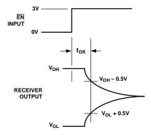
Figure 4. Receiver Disable Timing
