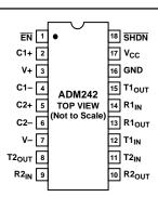
Figure 11. ADM242 DIP/SOIC Pin Configuration
