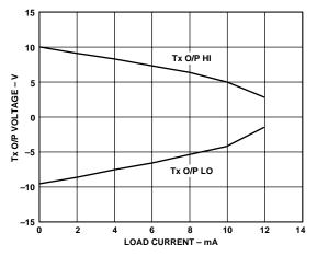
TPC 4. Transmitter Output Voltage vs. Current
