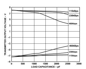
TPC 2. Transmitter Baud Rate vs. Load Capacitance
