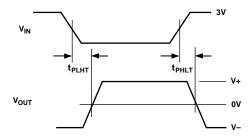
Figure 1. Transmitter Propagation Delay Timing
