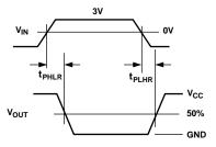
Figure 3. Receiver Propagation Delay Timing
