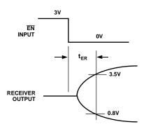
Figure 2. Receiver Enable Timing
