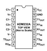
Figure 9. ADM232A DIP/SOIC Pin Configuration
