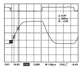
TPC 6. Transmitter Fully Loaded Slew Rate
