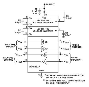
Figure 10. ADM232A Typical Operating Circuit
