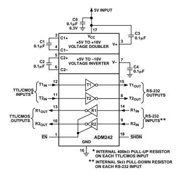
Figure 12. ADM242 Typical Operating Circuit
