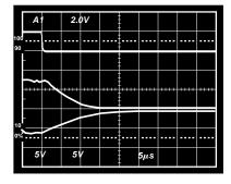
Figure 13. Transmitter Output Disable Timing
