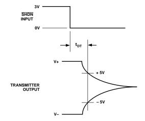
Figure 6. Transmitter Shutdown Disable Timing
