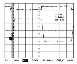
TPC 3. Transmitter Unloaded Slew Rate
