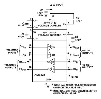
Figure 7. ADM222 Typical Operating Circuit
