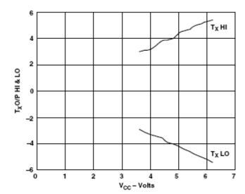
Figure 6. Tx Output Voltage vs. Supply
