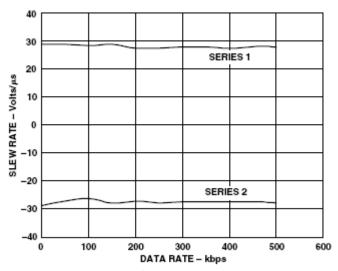
Figure 7. Slew Rate vs. Data Rate
