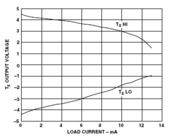
Figure 8. Transmitter Output Voltage vs. Load Current
