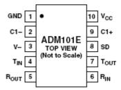
Figure 2. Pin Configuration
