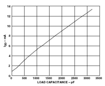
Figure 4. IDD vs. Load Capacitance at 460 kbps
