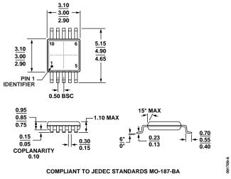
Figure 10. 10-Lead Mini Small Outline Package [MSOP] (RM-10) Dimensions shown in millimeters
