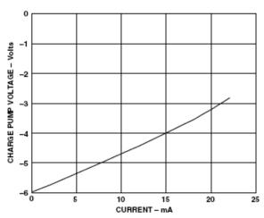
Figure 3. Charge Pump Voltage vs. Current
