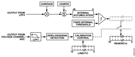
Figure 52. Reactive Energy Line Cycle Accumulation
