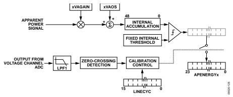
Figure 56. Apparent Energy Line Cycle Accumulation
