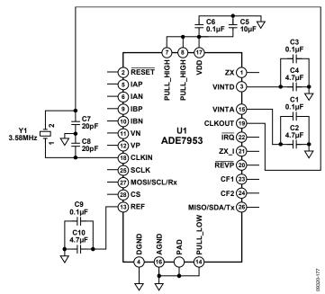
Figure 78. ADE7953 Crystal and Capacitors Connections
