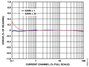
Figure 16. Current Channel A IRMS Error as a Percentage of Reading (Temperature =  $25^{\circ}$ C, Power Factor = 1) over Gain with Internal Reference, Integrator Off
