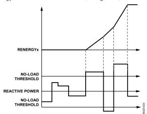
Figure 54. Reactive Energy Absolute Accumulation Mode
