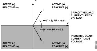
Figure 59. Capacitive and Inductive Loads
