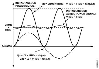
Figure 44. Active Power Calculation
