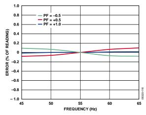
Figure 20. Current Channel B Active Energy Error as a Percentage of Reading (Gain = 1, Temperature = 25℃) over Frequency and Power Factor with Internal Reference, Integrator Off
