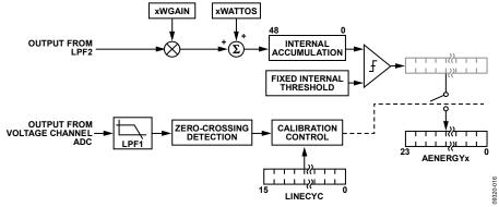
Figure 48. Active Energy Line Cycle Accumulation
