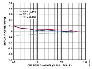
Figure 33. Current Channel B Reactive Energy Error as a Percentage of Reading (Gain = 16,  $Temperature = 25^{\circ}C$ ) over Power Factor with Internal Reference, Integrator On
