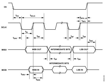
Figure 2. SPI Interface Timing
