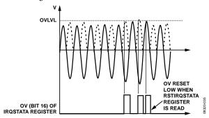
Figure 66. Overvoltage Detection
