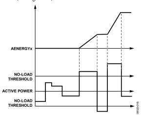
Figure 49. Positive-Only Accumulation Mode
