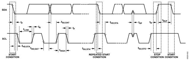
Figure 3. I<sup>2</sup>C Interface Timing
