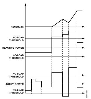
Figure 53. Reactive Energy Accumulation in Antitamper Accumulation Mode
