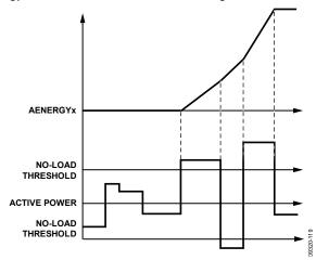
Figure 50. Active Energy Absolute Accumulation Mode
