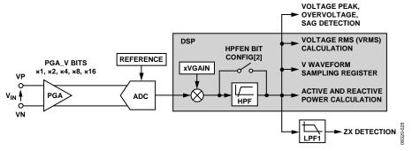
Figure 41. Voltage Channel ADC and Signal Path
