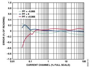
Figure 14. Current Channel A Reactive Energy Error as a Percentage of Reading (Gain = 22, Temperature = 25°C) over Power Factor with Internal Reference,
