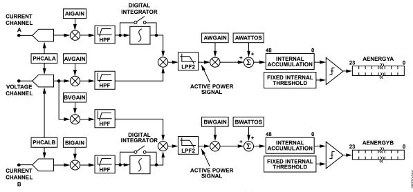
Figure 45. Active Energy Signal Chain
