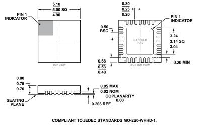
Figure 79. 28-Lead Lead Frame Chip Scale Package [LFCSP\_WQ]
