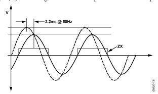
Figure 62. Voltage Channel ZX Output
