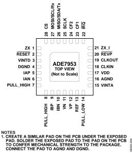
Figure 4. Pin Configuration
