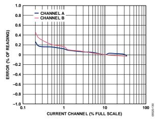
Figure 34. IRMS Error as a Percentage of Reading (Gain = 16, Temperature =  $25^{\circ}$ C) with Internal Reference, Integrator On
