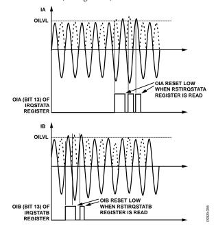
Figure 67. Overcurrent Detection
