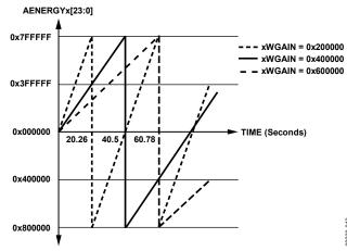
Figure 46. Energy Register Roll-Over Time for Active Energy
