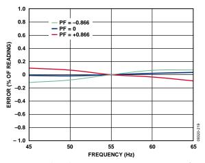
Figure 23. Current Channel B Reactive Energy Error as a Percentage of Reading (Gain = 1, Temperature = 25℃) over Frequency and Power Factor with Internal Reference, Integrator Off
