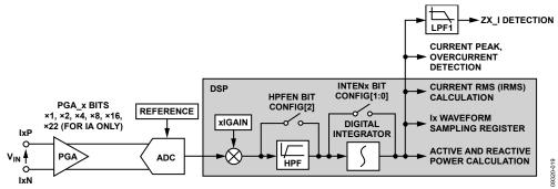
Figure 39. Current Channel ADC and Signal Path
