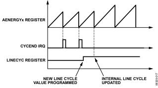
Figure 47. Changing the LINECYC Register
