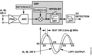
Figure 61. Zero-Crossing Detection
