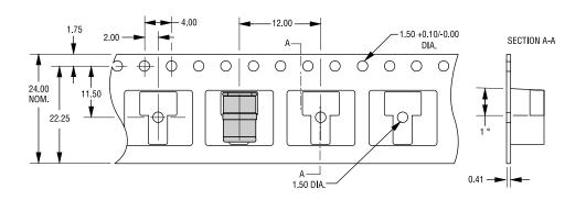
TOLERANCES: ±0.13 UNLESS OTHERWISE SPECIFIED DIMENSIONS: MILLIMETERS
