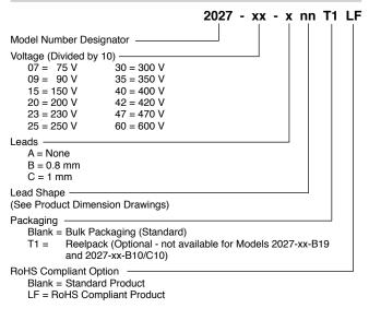
2027-XX-B - 0.8 ± .04 mm (0.032 ± 0.002 in.) dia. lead wire 2027-XX-C - 1.0 ± .04 mm (0.039 ± 0.002 in.) dia. lead wire
